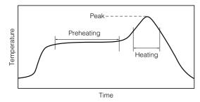
Recommended soldering conditions for flow
